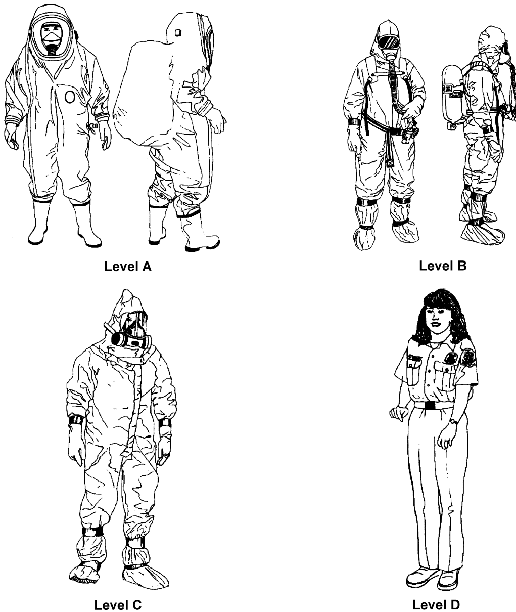
FIGURE 36-1. Levels of PPE. (From Agency for Toxic Substances and Disease Registry. Emergency Medical Services Response to Hazardous Materials Incidents. Available at: http://www.atsdr.cdc.gov/mhmi-v1-2.pdf .)
